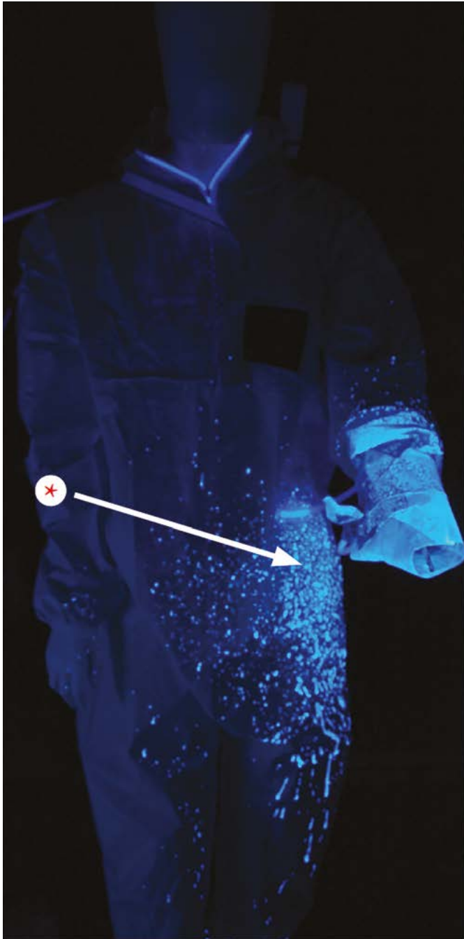
Figure 16: Shows a simulation of an operator using a compressed airline to remove MWF from a machined component, resulting in personal contamination with MWF droplets. The MWF was dosed with a blue dye, which under an ultra-violet lamp shows up as blue deposits on:
