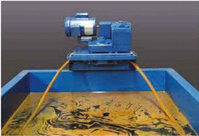
Figure 6b: Tramp oil (light brown) floating on the MWF surface.
