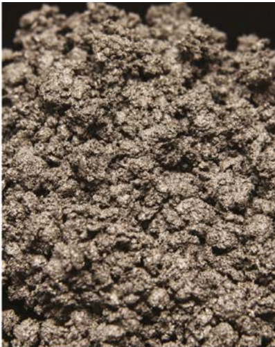
Figure 13b: Metal fines.
