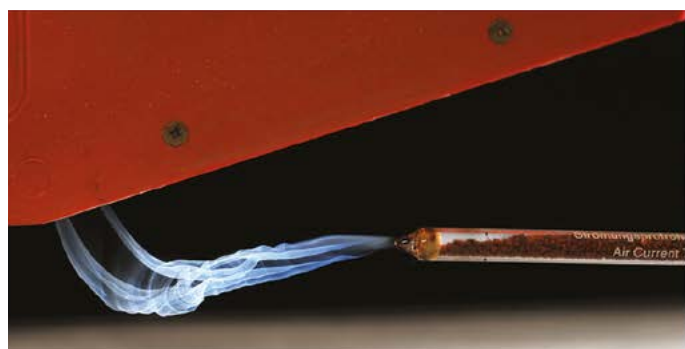
Figure 15a: Shows a smoke tube.
